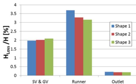
Figure 4. Loss analysis in the flow passage.
