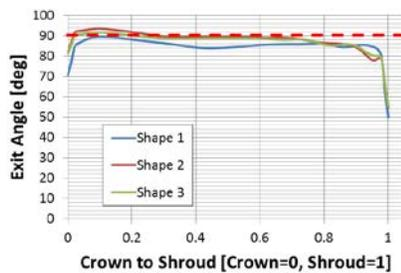
Figure 2. Exit angle from runner passage.
