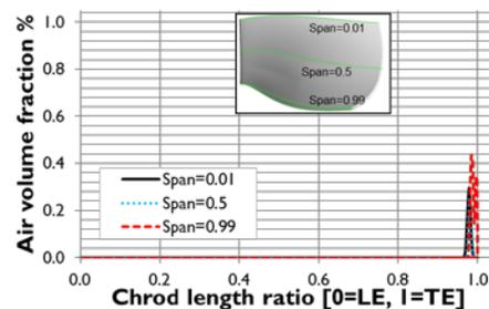
Figure 5. Cavitation analysis result
