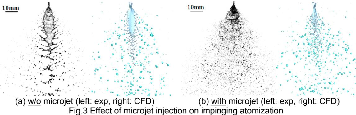
Fig.3 Effect of microjet injection on impinging atomization
