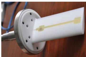
Figure 1. Cantilevered flexible hydrofoils used for vibration and strain measurements.
