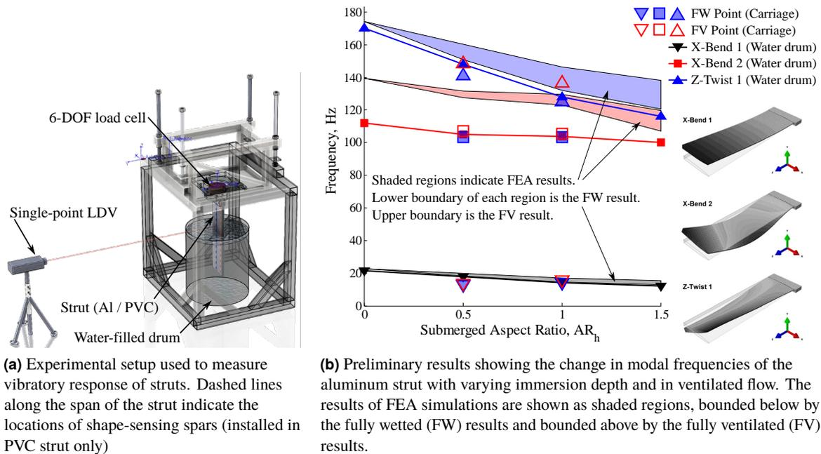
**Figure 1.** The experimental setup is depicted in (a). Preliminary results for the Aluminum strut are shown in (b).
