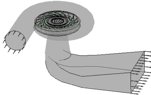
Figure 1. The whole model of passage flow(include clearance)
