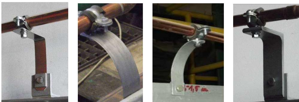
**Figure 2** The pipe fixed with various types of flat springs (from the left: FS2, FS3, FS4, FSR)
