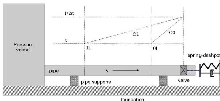
Figure 1. Physical model of the pipeline with viscoelastic valve attachment
