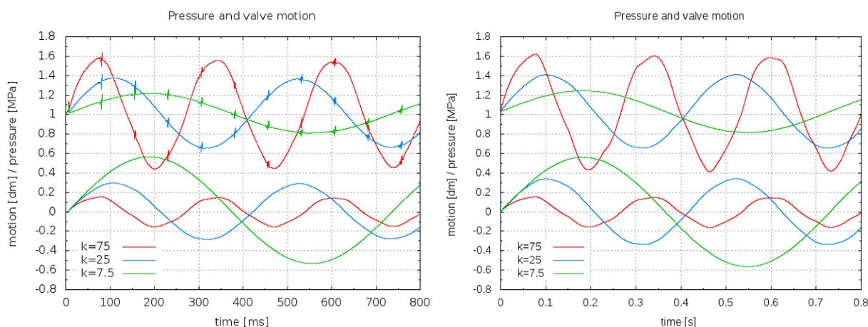
**Figure 2** Numerical (left) and analytical (right) results of the pressure records (upper plots) and axial valve motions (lower plots) for small stiffness ( $k$ ) of the valve spring
