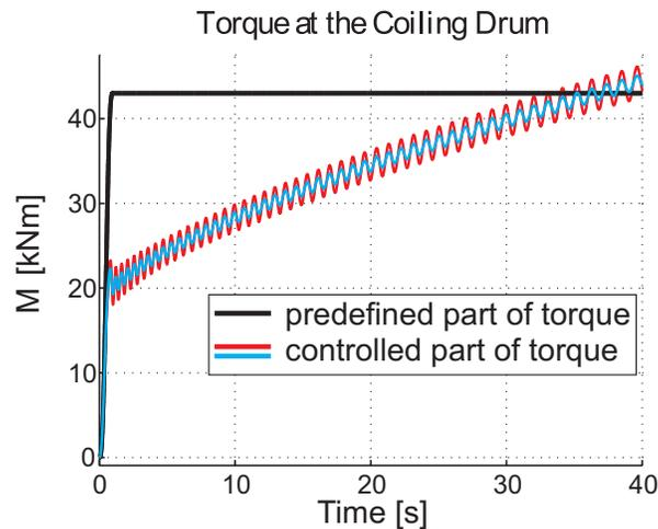
**Figure 1.** Torque at the rotor for a constant axial speed.
