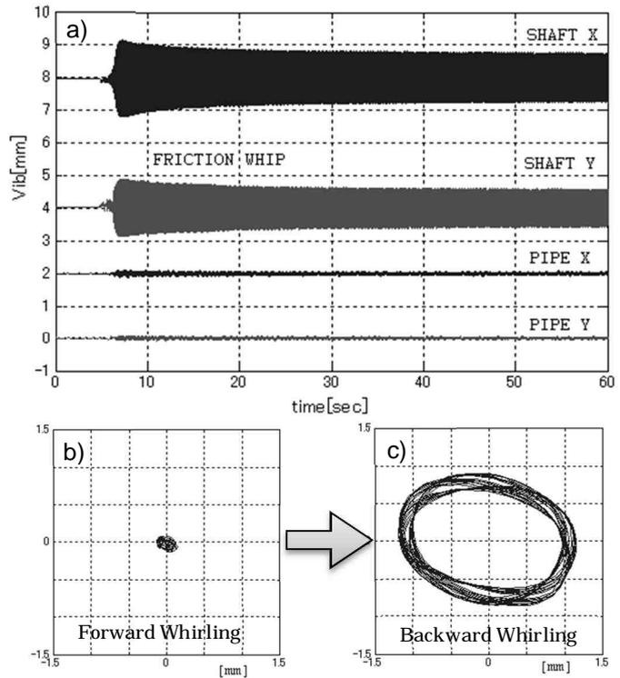
Fig.2 An Example of Friction Whip
