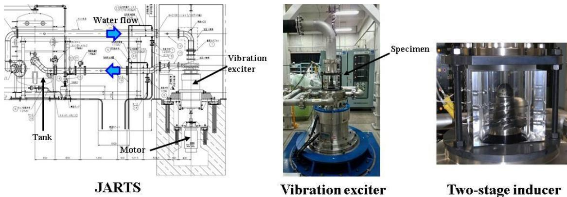
Figure 1. Schematic of JARTS and the test configuration
