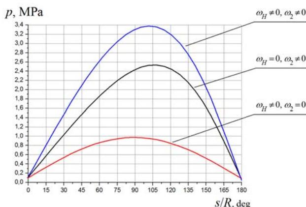
Figure 2. Pressure distribution in bearing middle section for different planet wheel rotation conditions
