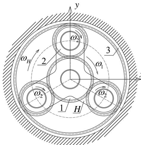
**Figure 1.** Planetary gear
