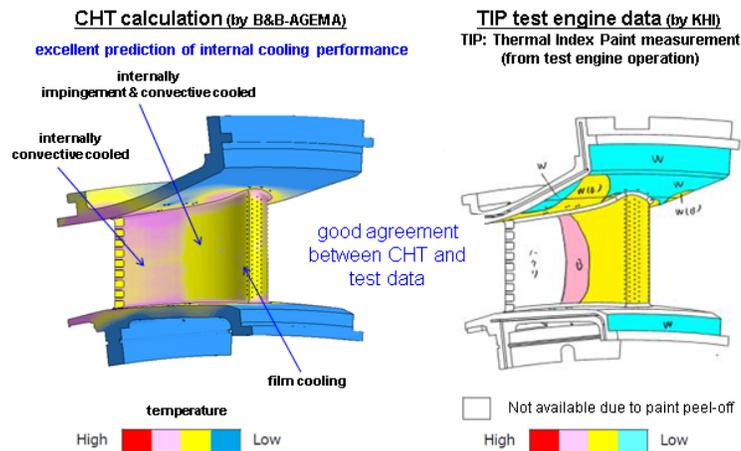
Figure 1. Example results for comparison of thermal load
