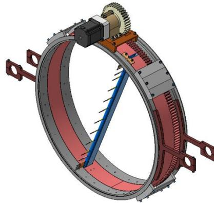
Figure 5. Design of the traversable measurement rake
