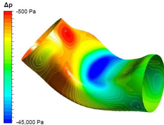
Figure 4. Forces acting on the duct structure
