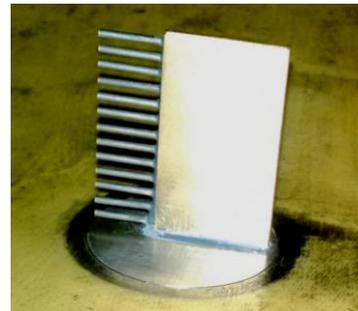
Figure 3. Boundary layer probe
