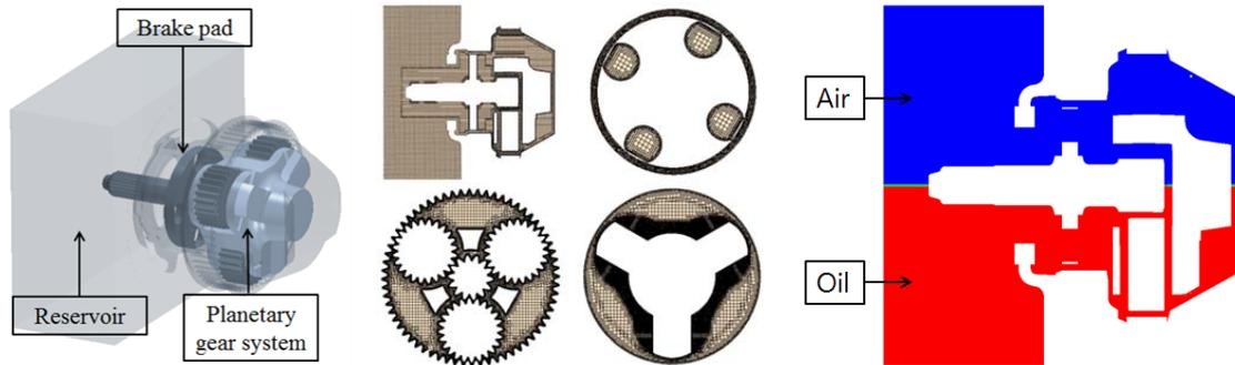
Figure 1. Schematic view of transaxle brake and boundary condition.
