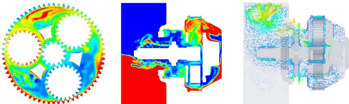
Figure 2. Oil volume fraction and velocity vector plot inside of the brake at quasi-static state.
