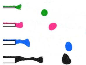
**Figure 4.** Effect of atomizing edge thicknesses on droplet size
