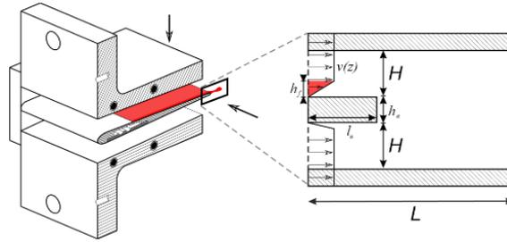
**Figure 1.** Flat air blast atomizer test section
