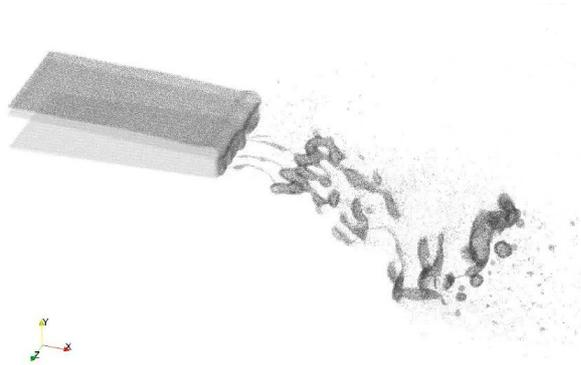
**Figure 3.** Snapshots of air blast atomization as predicted by the SPH method
