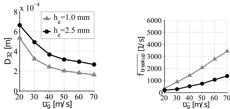
**Figure 2.** Effect of atomizing edge thickness droplet size and detachment frequency
