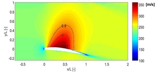
**Fig.3** Velocity contours around blade.
