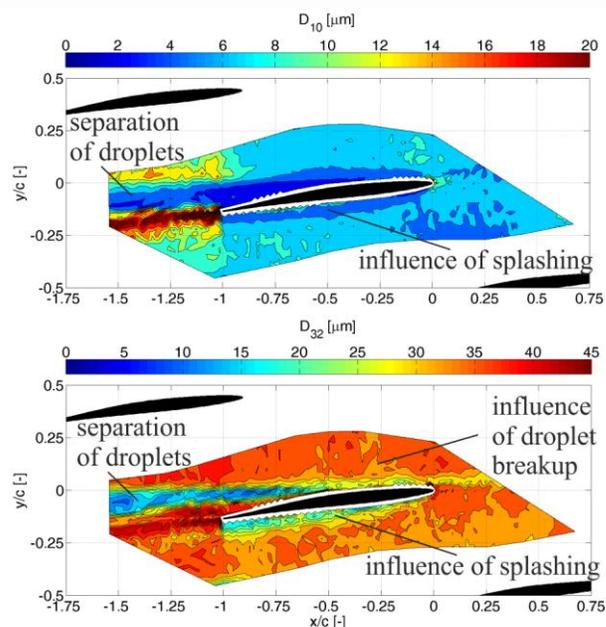
**Fig. 1** Contour plot of  $D_{10}$  and  $D_{32}$  around a transonic profile at a water load  $\xi_w=1.3\%$ ,  $Ma_1=0.89$  and inlet flow angle  $\beta_1=153^\circ$  [4].
