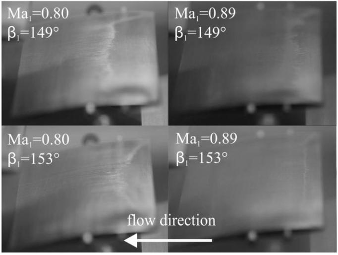
**Fig. 2** Wall film pattern at  $\xi_w=1.3\%$ ,  $Ma_i=0.80$  (left) and  $Ma_i=0.89$  (right) at  $\beta_i=149^\circ$  (top) and  $\beta_i=153^\circ$  (bottom) [4].
