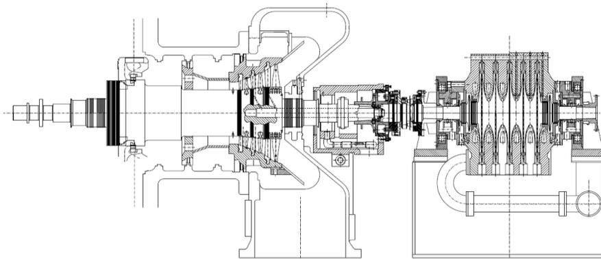
Figure 1. Full-scale industrial steam turbine test facility at ITSM
