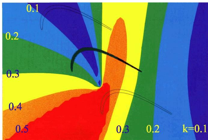
Figure 1, Critical Reduced Frequency as a Function of Pitching Axis Location
