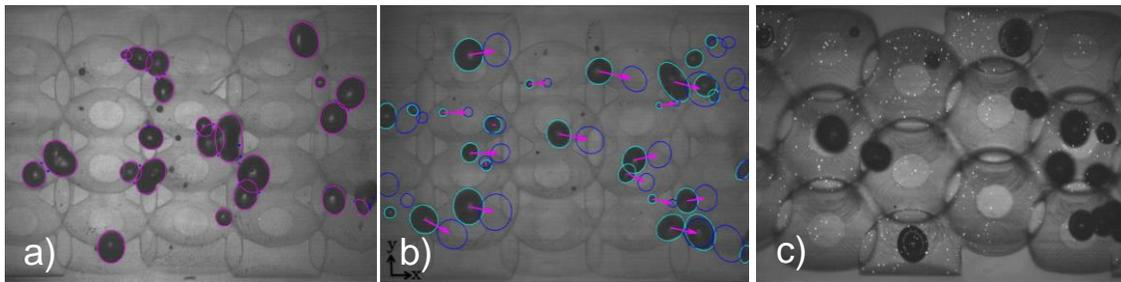
**Figure 2.** a) Bubble detection by ellipse fitting b) Bubble tracking c) PSI and PPIV
