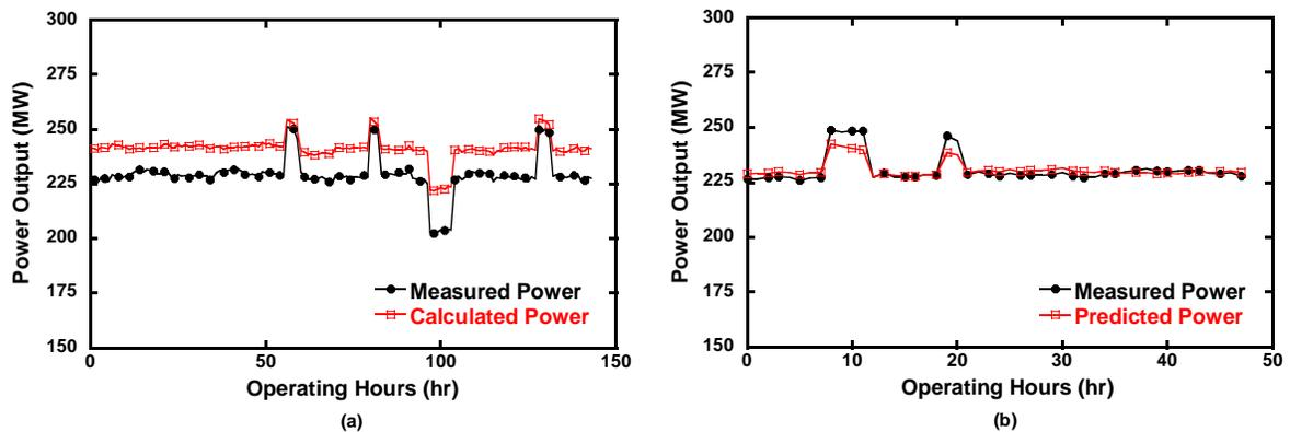
Figure 3. Comparison and validation of the methodology : (a) calculated and measured powers, (b) predicted and measured powers
