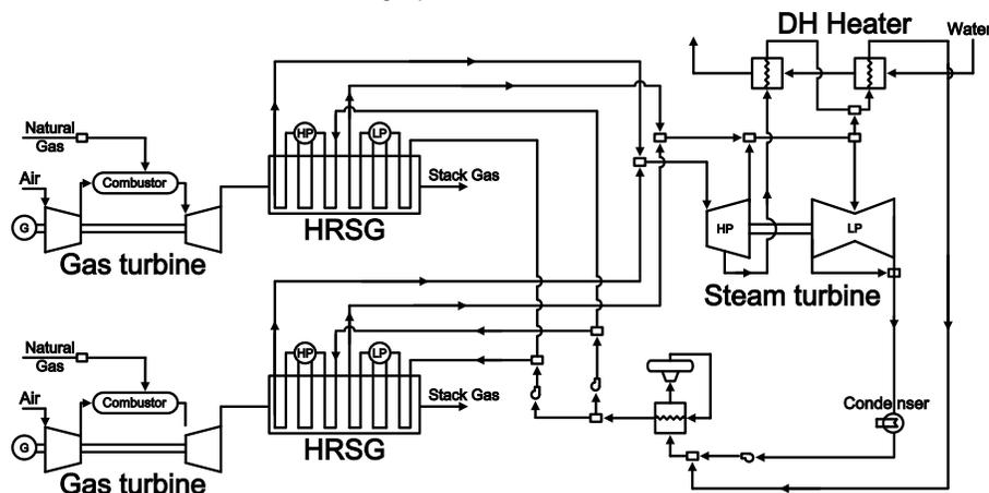
Figure 1. Configuration of the combined cycle cogeneration plant
