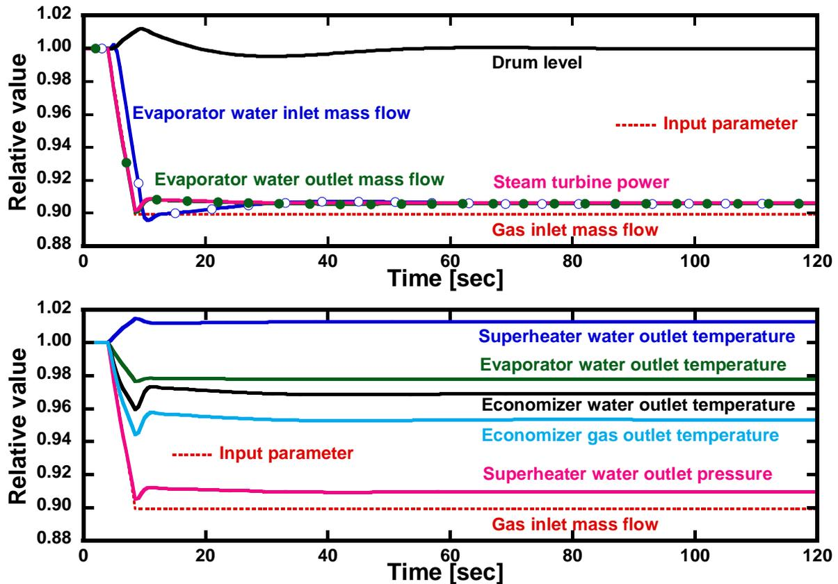
Figure 1. Dynamic simulation results of a single pressure bottoming cycle
