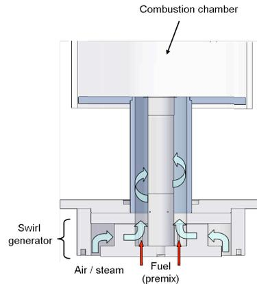
Figure 1. The injector
