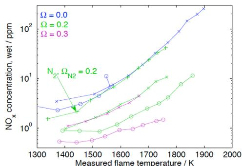
Figure 3: Measured NO<sub>x</sub> concentration versus measured flame temperature for natural gas (—x—) and hydrogen (—o—). The equivalence ratio was decreased from  $\phi = 0.95$  (dry H<sub>2</sub> flame from  $\phi = 0.55$ ) to blowout for each curve ( $T_{in} = 623$  K).
