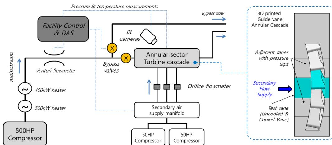
Figure 1. Schematic view of transonic turbine cascade facility and test cascade
