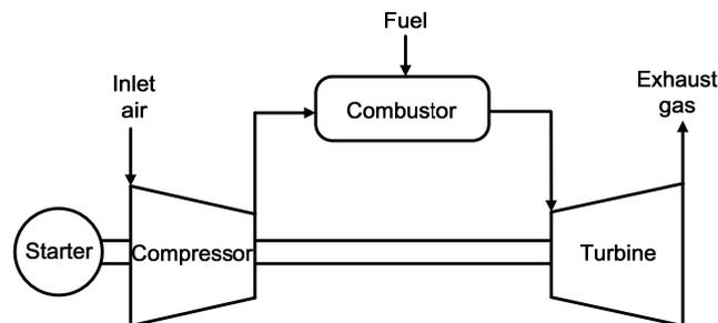
Figure 1. Gas turbine configuration
