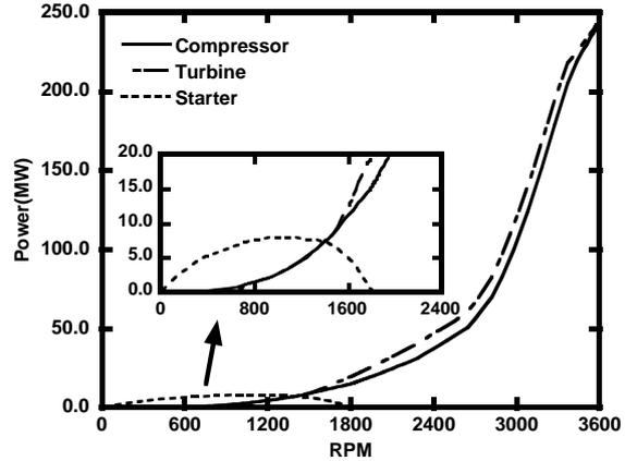
Figure 3. Components power during start-up
