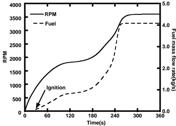
Figure 2. Fuel scheduling and gas turbine speed response during start-up
