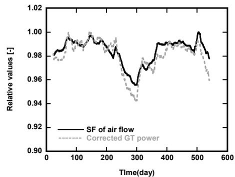
**Figure 4.** Comparison of relative values of corrected GT power output and SF of air flow
