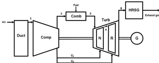
Figure 1. Layout of the gas turbine
