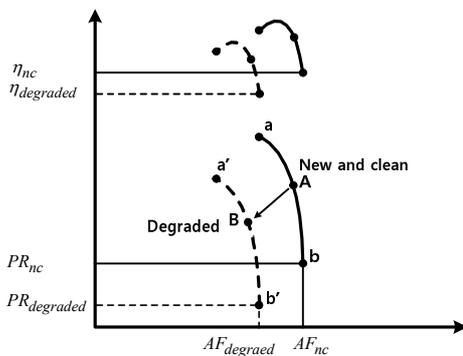
**Figure 3.** Adaptive method of compressors map
