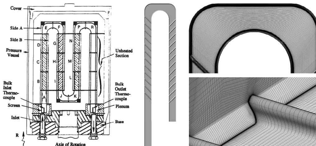
Figure 1. Four-pass cooling channel by Johnson et al. [2] and modeled two-pass channel with two numerical grid detail views
