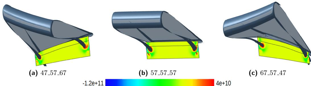
**Figure 2.** Visualisation of clearance vortices - isosurface at  $5 \cdot 10^{10}$  and contour of the Q criterion for configurations based on the nominal case.
