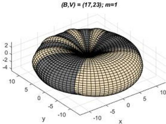
**Figure 1.** Free-field directivity pattern of the disturbed rotor-stator WIN at the BPF. Fan axis along the vertical direction, pointing at inlet.
