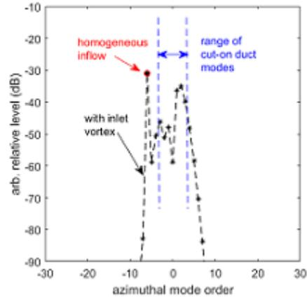
**Figure 2.** Envelope of the free-field azimuthal modal spectrum of WIN at the BPF for a far-field observer at  $30^\circ$  from axis..
