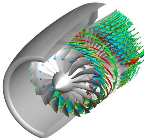
**Figure 3.** Iso Q-criterion for the turbofan configuration
