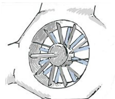
**Figure 1.** Advanced shrouded tail-rotor viewed from downstream. Leaned vanes in grey and unevenly-spaced rotor blades in light blue.
