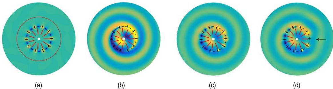
**Figure 3.** Examples of modal fields synthesized by discretized source modes. (a),(b): modes  $s=0$  and  $s=1$  of the homogeneous stator noise, parameters given in the text. (c),(d): full stator noise of the homogeneous and actual (with 1 vane removed from 11; case of Figure 1) systems.
