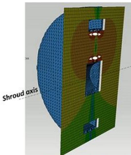
**Figure 4.** Computed sound-pressure amplitude map in the meridian plane (Figure 2) for two point dipoles in the plane located close to the hub and close to the shroud.
