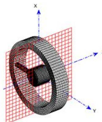
**Figure 2.** Simplified shroud for scattering computations, transmission shaft, and main axes for the modeling. Meridian cut in red.
