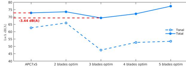
**Figure 1.**  $L_{wA}$  for the reference and the optimized blades
