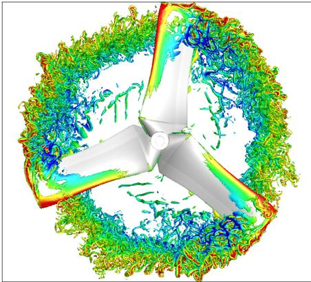
**Figure 2.** Iso-surface of the Q-criterion on the optimized blade.
