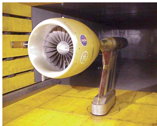
Figure 1. Source Diagnostic Test test rig at NASA Glenn Low Speed Wind Tunnel
