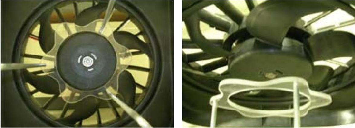
**Figure 1.** Wavy obstruction in front of an axial engine cooling fan (Gerard, 2009)
