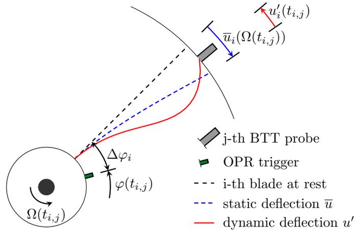
**Figure 1.** Sketch of the  $i$ -th Blade Tip Arriving at  $j$ -th BTT Probe at time  $t_{i,j}$
