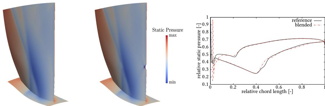
**Figure 1.** Comparison of Static Pressure for Reference Geometry and Blending Repaired Blade
