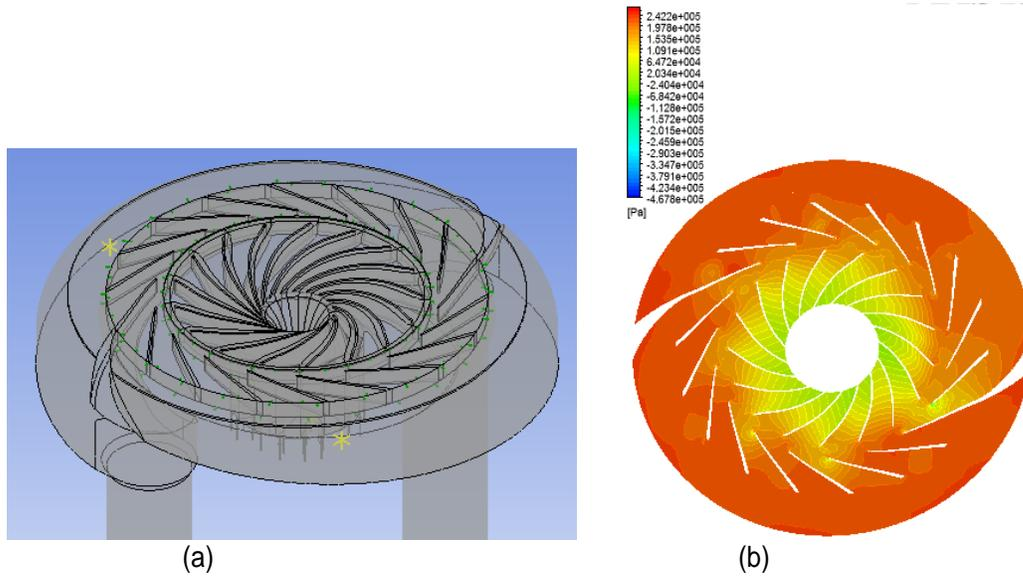
**Figure 2** 3-D CFD calculation result.
