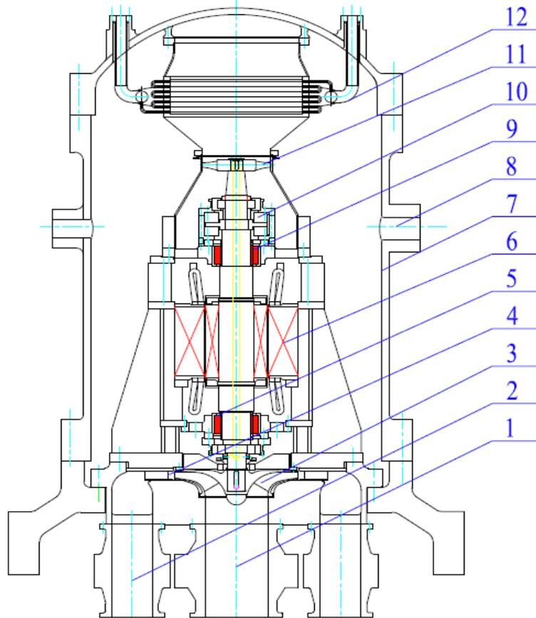
1. Inlet Valve, 2. Outlet Valve, 3. Impeller, 4. Diffuser, 5. Lower Radial Magnetic Bearings, 6. Motor, 7. Pressure Vessel, 8. Electric Penetration, 9. Upper radial Magnetic bearings, 10. Axial Magnetic Bearing, 11. Cooling Impeller, 12. Motor Cooler.
