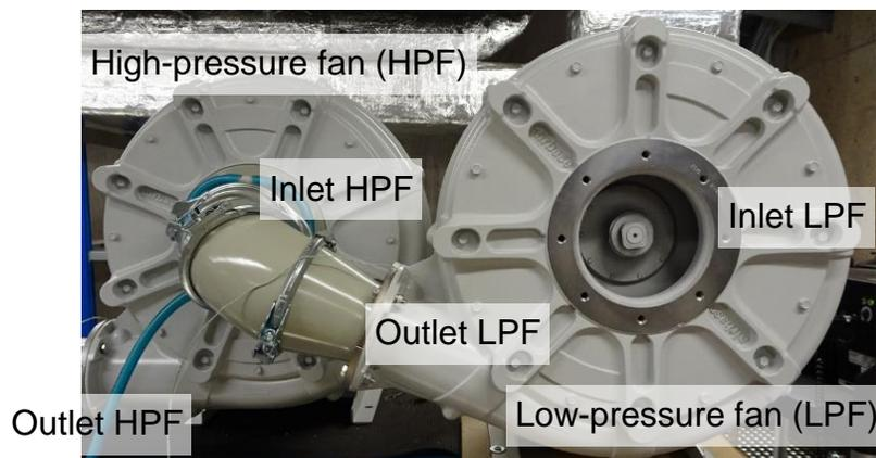
Figure 1. Serial arrangement of two centrifugal fans
