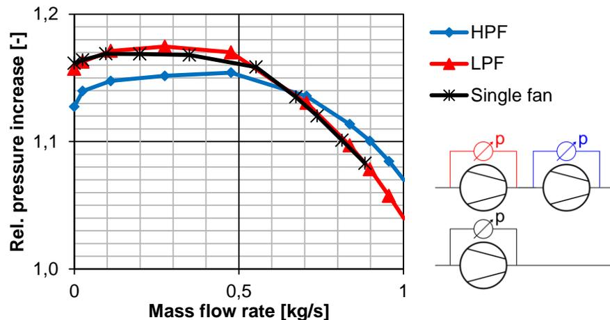
Figure 2. Relative pressure increase over volume flow rate
