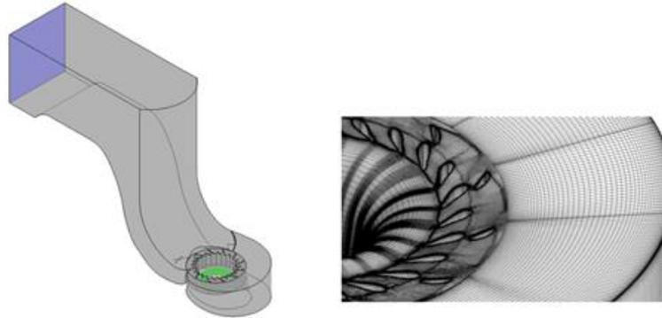
**Figure 1.** Computational domain (left) and mesh in the distributor and semi-spiral case (right). The inlet is shaded with light blue color and the outlet with the light green color in the left figure.
