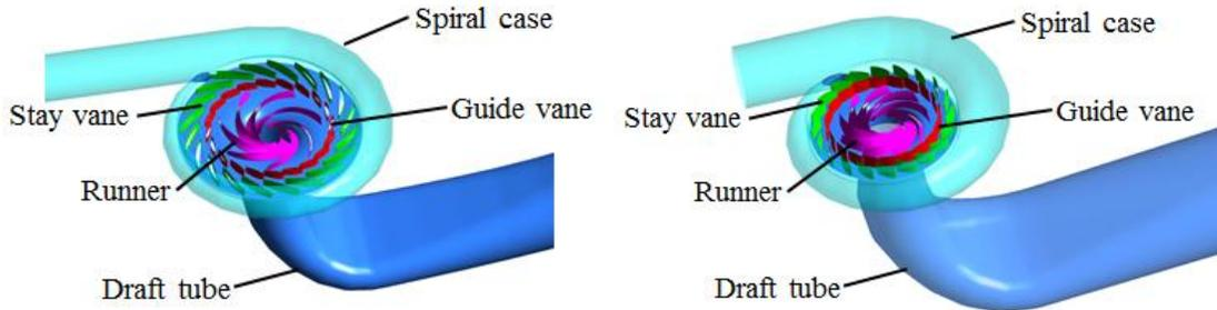
Figure 1. CFD computational domain of the pump turbine
