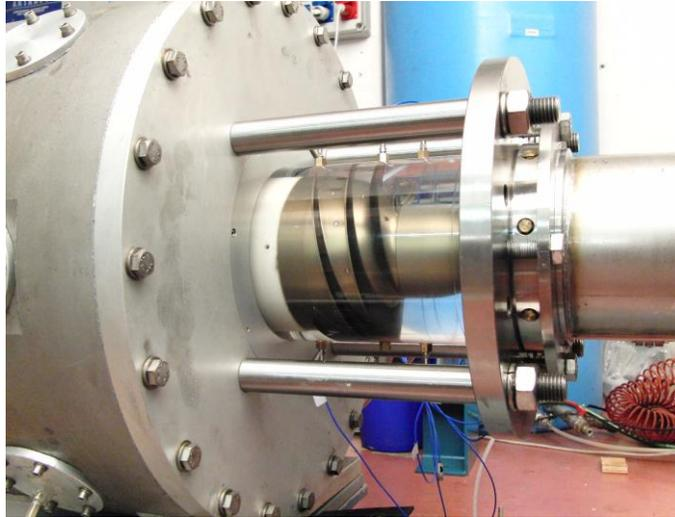
**Figure 1.** Test Section of the Cavitating Pump Rotordynamic Test Facility at SITAEL S.p.A.
