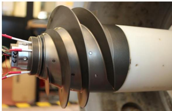
**Figure 2.** The RAPDUD inducer equipped with pressure taps along the blade channels.
