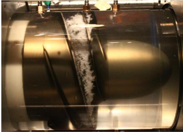
**Figure 2.** A picture of the RAPDUD inducer under cavitating conditions.
