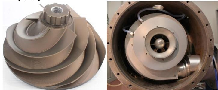
Figure 3. Centrifugal impeller (left) and test assembly (right).
