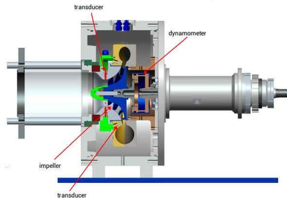
Figure 2. 3D cut-off with a sample of the transducer positions for instabilities characterization.
