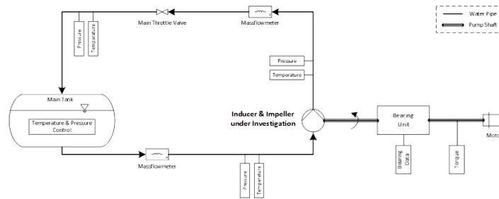
**Figure 1.** Schematic drawing of the designed water test bench.
