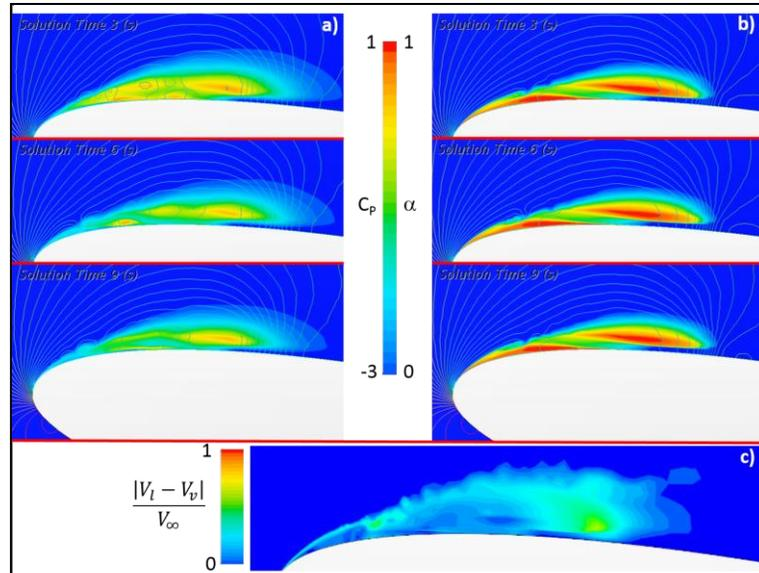
**Figure 1.** Comparison of a) homogeneous, b,c) 2-Fluid cavitation predictions for a NACA 0012,  $\alpha=10^\circ$ ,  $Re_c=5 \times 10^6$ ,  $\sigma=2.4$ . a,b) contours of  $C_p$  and gas volume fraction at three corresponding timesteps. c) normalized slip velocity at a given timestep.
