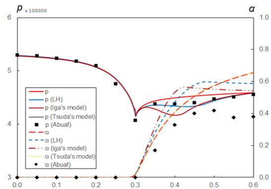
**Fig.2** Comparison of pressure and void fraction along nozzle three models and Abuaf's results in case  $T=422.5\text{K}$
