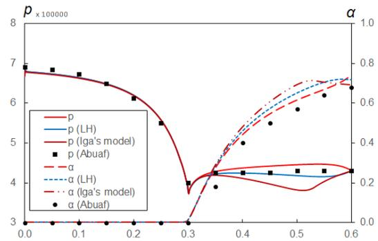
**Fig.1** Comparison of pressure and void fraction along nozzle three models and Abuaf's results in case  $T=421\text{K}$
