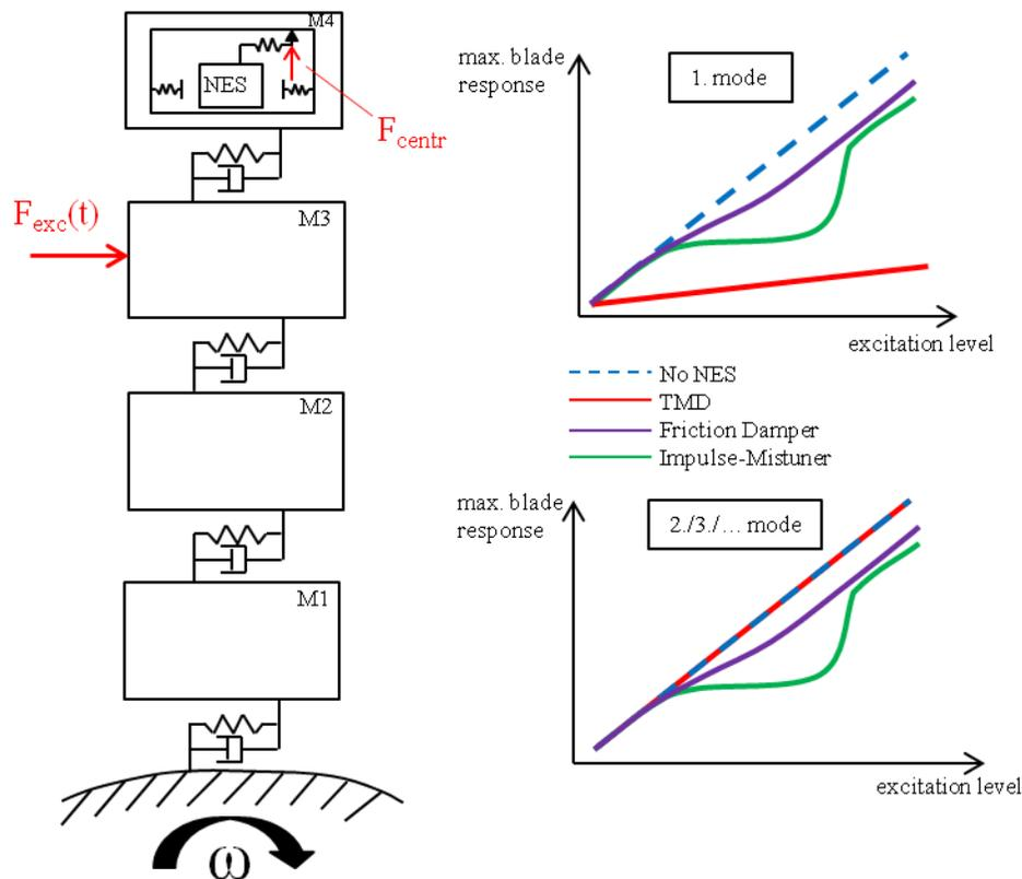
**Figure 1:** Model (left) and absorber effectiveness for various modes compared to tuned mass damper and friction damper (right)
