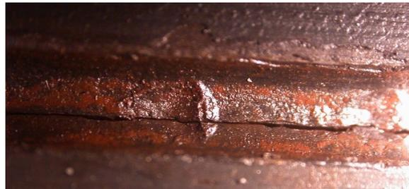
**Figure 1.** Initiation points in the dovetail slots of 1<sup>st</sup> high pressure stage and crack close-up.
