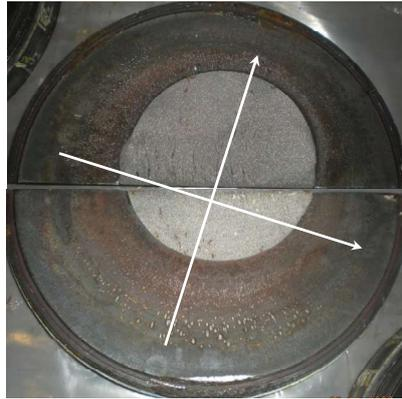
**Figure 2.** Front view of the complete cracked section of the shaft.
