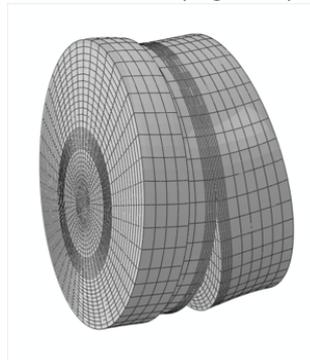
**Figure 3.** Detail of the 3D finite element model of a short part of the shaft that contains the cracked section.
