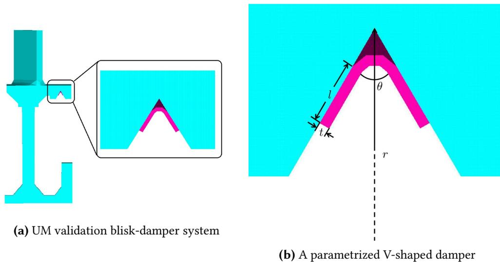
**Figure 1.** A typical blisk-damper system: UM validation blisk (blue) in contact with a V-shaped ring damper (purple). The damper is parametrized into four geometric parameters.
