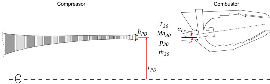
**Figure 1.** Compressor and combustor interface parameter.
