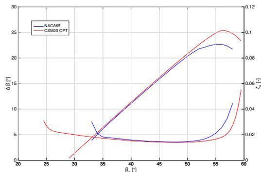
**Figure 2.** Flow turning and loss coefficient
