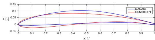
**Figure 1.** Profile geometry comparison
