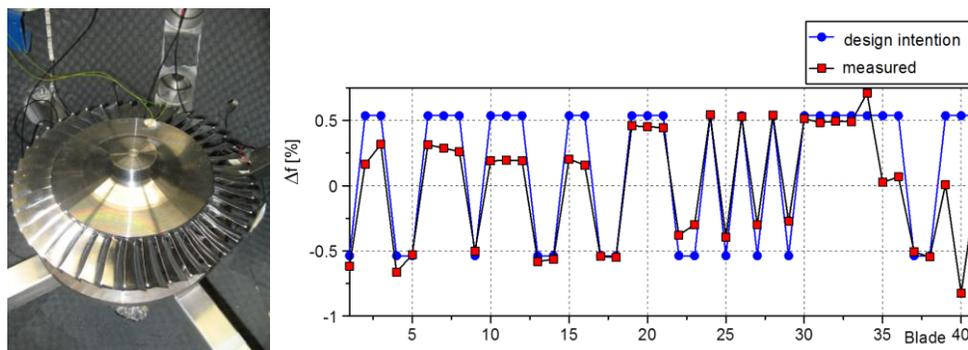
**Figure 1.** Blisk prototype (left) and frequency mistuning of fundamental flap mode (right)
