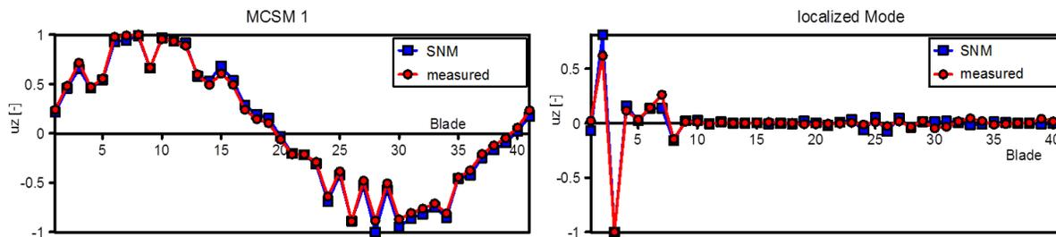
**Figure 2.** Measured and computed mode shape involutes (M1/leading edge tip)
