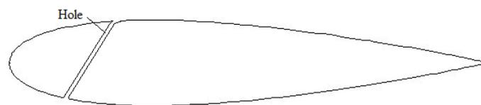
Figure 1. Schematic of the modified aerofoil geometry
