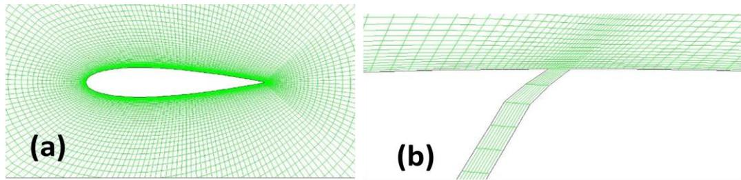
Fig. 1. (a) Mesh around the aerofoil. (b) Zoomed view near the opening of the hole.
